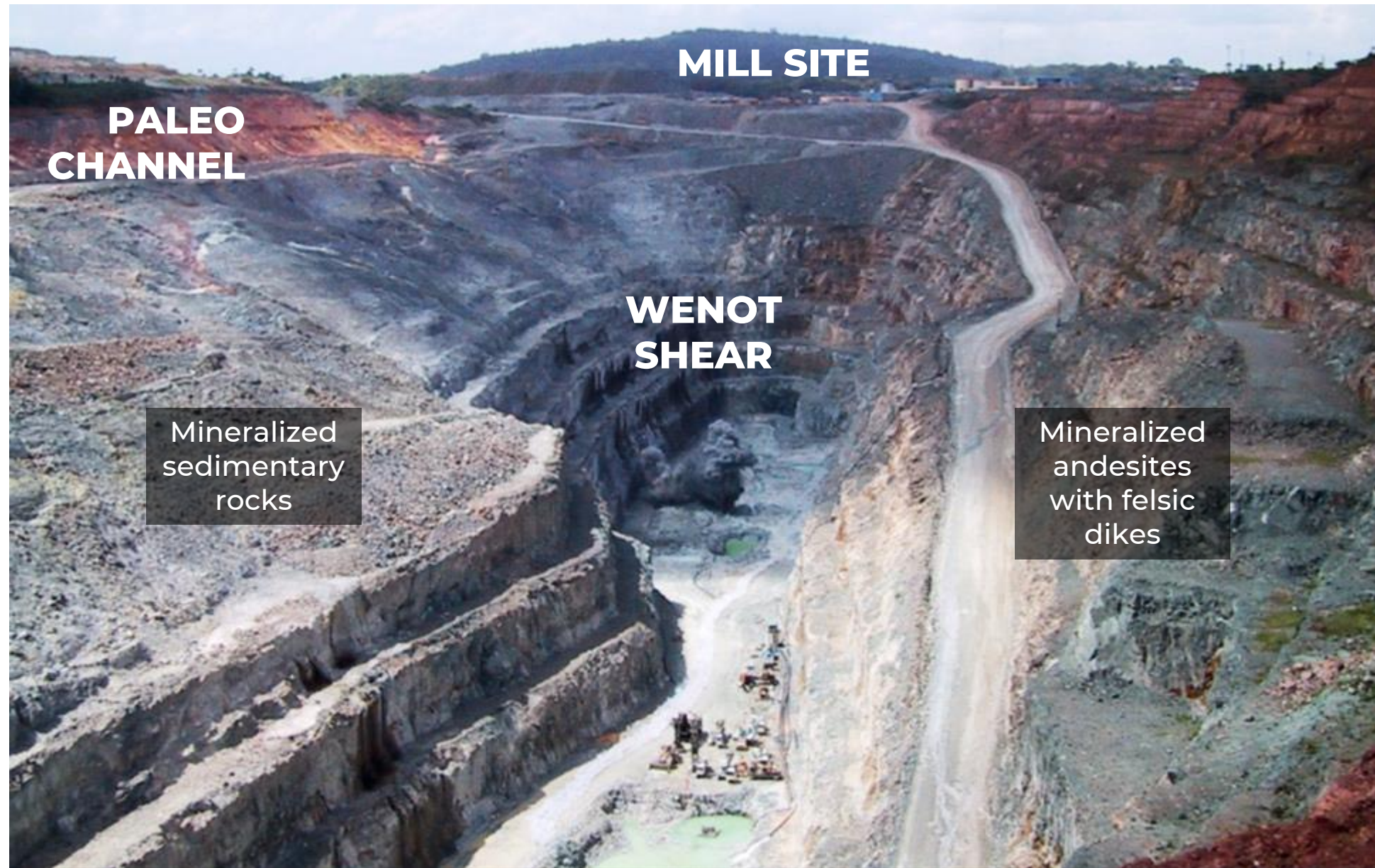
Photo looking west. High-grade complex shear with felsic dikes was mined. Mineralization continued under the mill site and recent drilling indicates gold in sediments and andesites
